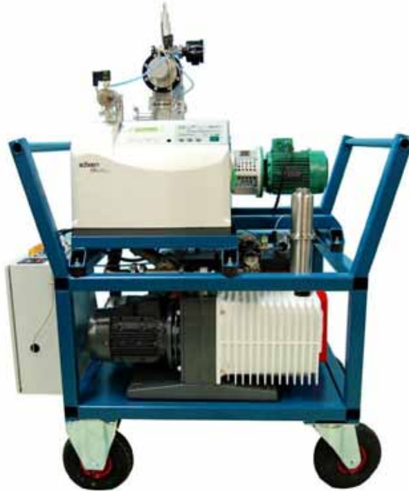
FIG. 1.10. Portable Helium Leak Testing System.
