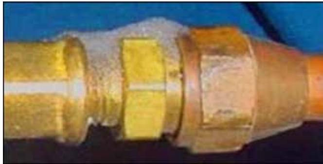
FIG. 3.1. Foam film to detect gas bubbles.
