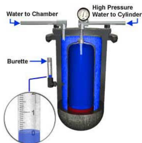
FIG. 6.1. Water jacket test.
