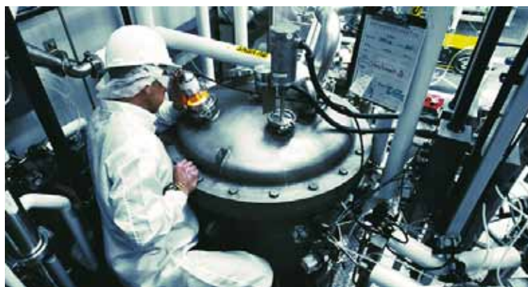
FIG. 3.5. Portable He leak tester being used in pharmaceutical industry.
