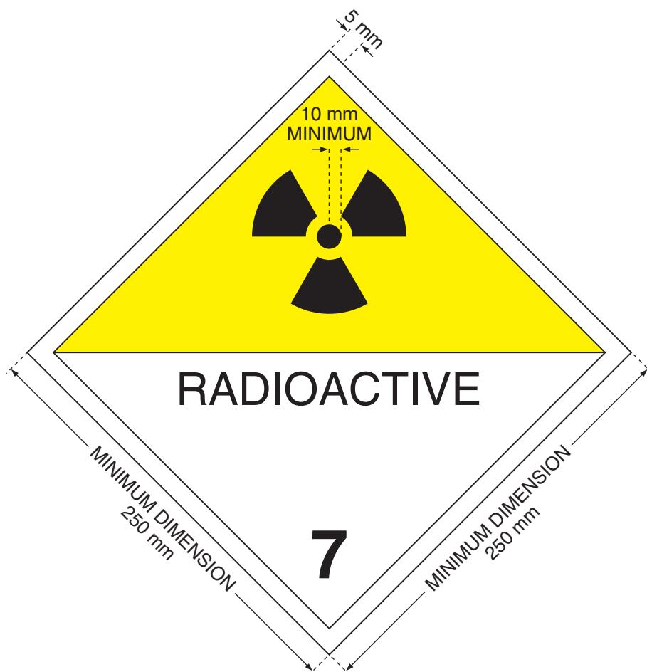
FIG. 6. Placard. Except as permitted by para. 571 minimum dimensions shall be as shown; when different dimensions are used the relative proportions must be maintained. The number '7' shall not be less than 25 mm high. The background colour of the upper half of the placard shall be yellow and of the lower half white, the colour of the trefoil and the printing shall be black. The use of the word "RADIOACTIVE" in the bottom half is optional to allow the alternative use of this placard to display the appropriate United Nations number for the consignment.
